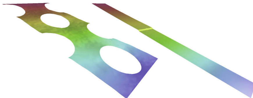
Fig. 10. Comparison of a material with voids (left) to a homogeneous strip (right) at t = 3.75 . The homogeneous strip shows a wavefront still present. Reflections and diffraction due to the voids, in combination with intrinsic diffusion, eliminate the wavefront in the perforated material.
