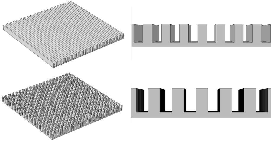
Figure 1: 2D and 3D Pristine Base Micro-structures for Optimization
