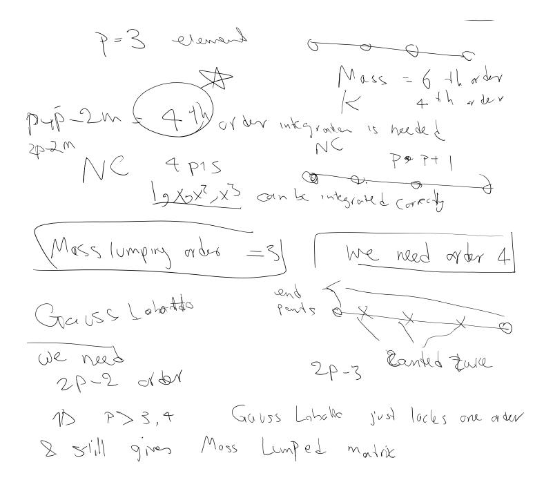
If reduced order quadrature is used, we need to enforce condition (a) above to ensure preserving the maximum convergence rates for modal quantities and enforce condition (b) to ensure convergence of modal quantities to exact values as  $h \rightarrow 0$  (the minimum requirement)
