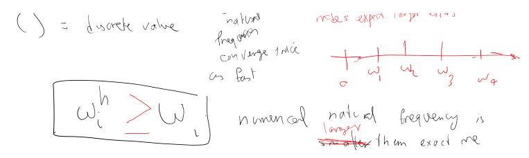
grid resolution h = the largest element size (size of an element is the radius of its circumscribing circle (2D) / sphere (3D)) 1.  $0 \le \omega_i^h - \omega_i$ , *i.e.*, having  $\omega_i^h \le \omega_i$  is not preserved once the Galerkin rules are violated [Hughes, 2012] (e.g., when reducedintegration or incompatible modes are employed or when lumped mass matrix is used).
