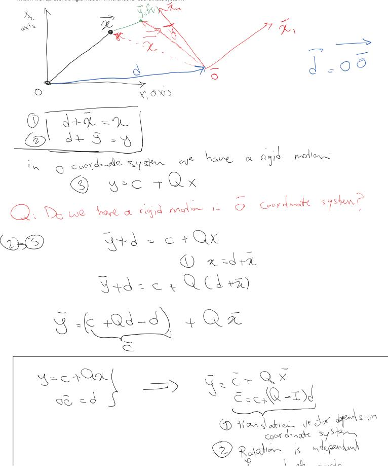
Kinematics: Change in length, angle, area, and volume by deformation We first study these changes for finite deformation and eventually find their approximate form for infinitesimal deformation
