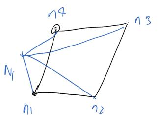
Even if we form shape functions in real geometry the integration of element stiffness matrix is very difficult in this geometry ->
