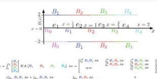
$$K = \int_{0}^{2} \begin{bmatrix} B_{1} \\ B_{2} \\ B_{3} \end{bmatrix} EA \begin{bmatrix} B_{1} \\ B_{2} \end{bmatrix} B_{1} dx = \begin{bmatrix} \int_{0}^{2} B_{1} B_{1} dx & \int_{0}^{2} B_{1} B_{2} dx & \int_{0}^{2} B_{1} B_{3} dx & \int_{0}^{2} B_{1} B_{3} dx & \int_{0}^{2} B_{2} B_{3} dx & \int_{0}^{2} B_{3} B_{3} dx &$$
