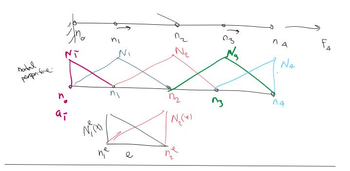
Calculating the stiffness matrix using the element-centered approach:
