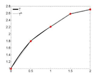
u<sup>h</sup> and u match at all nodes n<sub>0</sub>, n<sub>1</sub>, n<sub>2</sub>, n<sub>3</sub>, and n<sub>4</sub>. This holds for 1D solid elements with uniform AE and does not hold in general.
