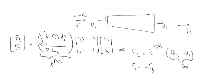
KFEM stiffeness is not exact for AE = constant x=L Uz Exact solution
