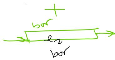
$$K_{beam} = \frac{AE}{l_2} \begin{bmatrix} 1 & -1 \\ -1 & 1 \end{bmatrix}$$
