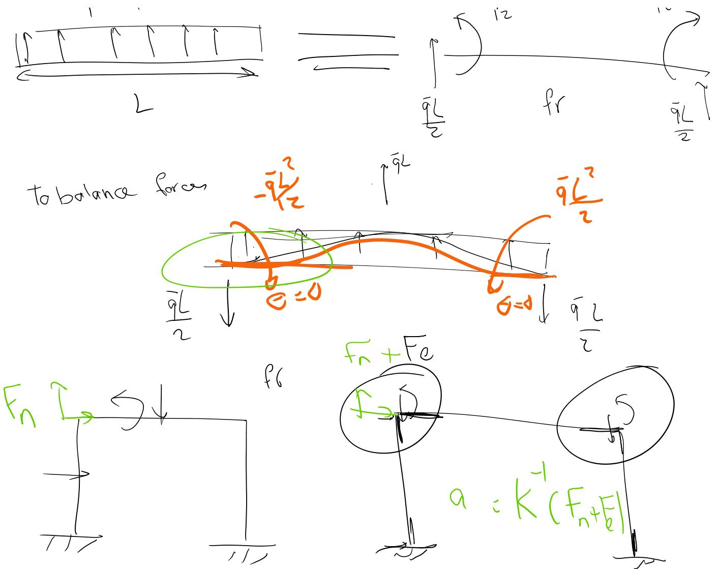
5. **80 Points** In figure 5 Frame element  $e_2$  is hinged to truss element  $e_1$ . For the frame element, a concentrated moment  $\bar{M} = 1$  is applied at  $x = 0.75$  and a distributed load  $q = x$  is applied over the length of the frame.
