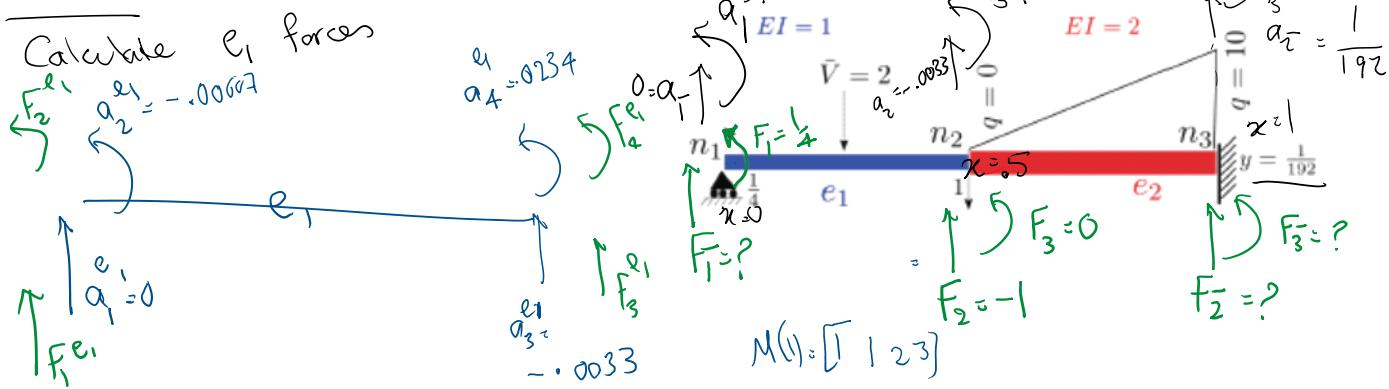
$$f_D^{e_1} = k_{4 \times 4}^{e_1} a_{4 \times 1}^{e_1} = k^{e_1} \begin{bmatrix} 0 \\ -0.00607 \\ -0.00332 \\ 0.023434 \end{bmatrix}$$
