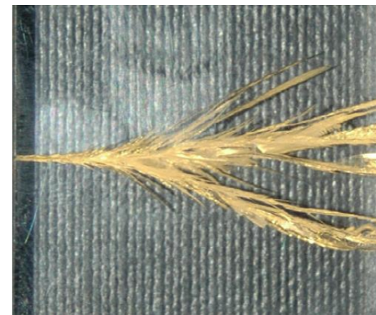
DynamicFractureBifurcation PMMA Murphy 2006
