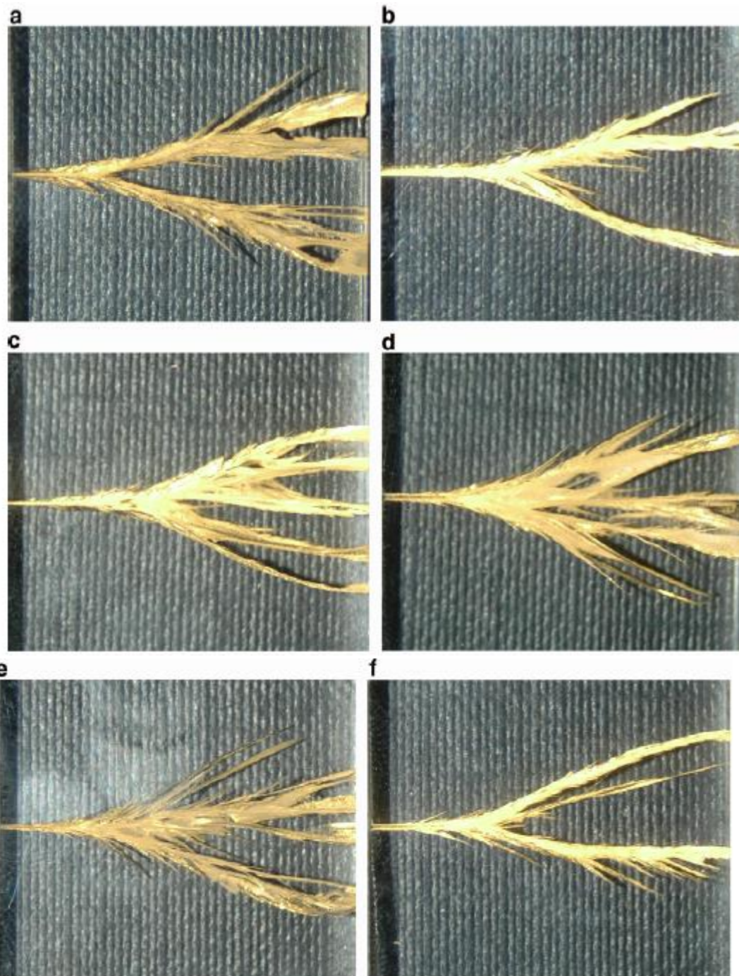
Fig. 5. Macroscopically planar fracture surfaces for the specimens containing the (a) 2.0 mm, (b) 1.4 mm, (c) 1.0 mm and (d) 0.5 mm notches.
