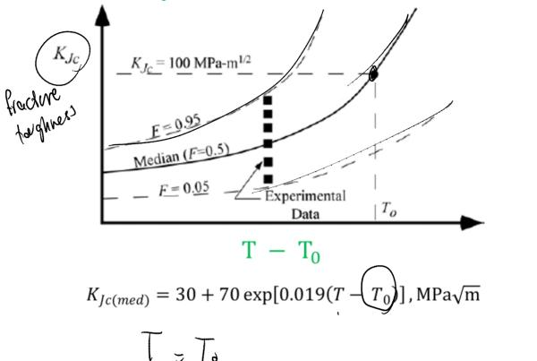
Irradiation increases TO and shifts the curve to the right (meaning the material becomes more brittle)
