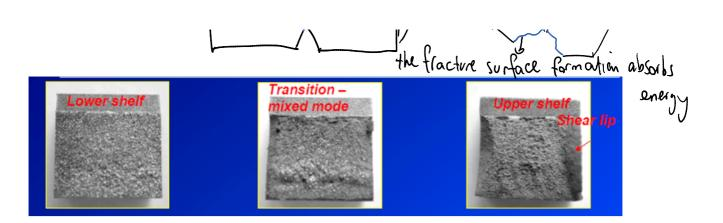
Energy loss:  $mg(y_z-y_i) = fracture energy for_E$ the specimen
