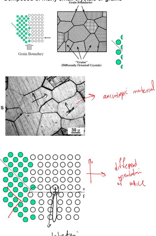
How does the grain size change the ductility and strength of a material?
