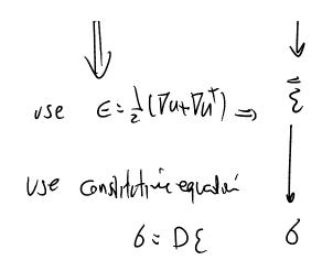
Second approach: we use it to solve the stress field for modes I and II crack (tip) stress fields
