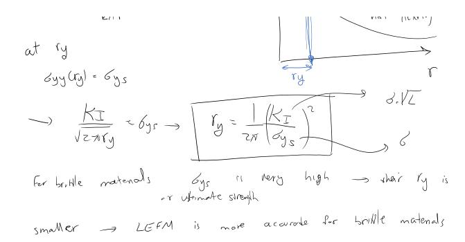
The problem with this model is that stress is not redistributed (we really have to solve the crack tip fields by using a material that from beginning of the analysis can yield)
