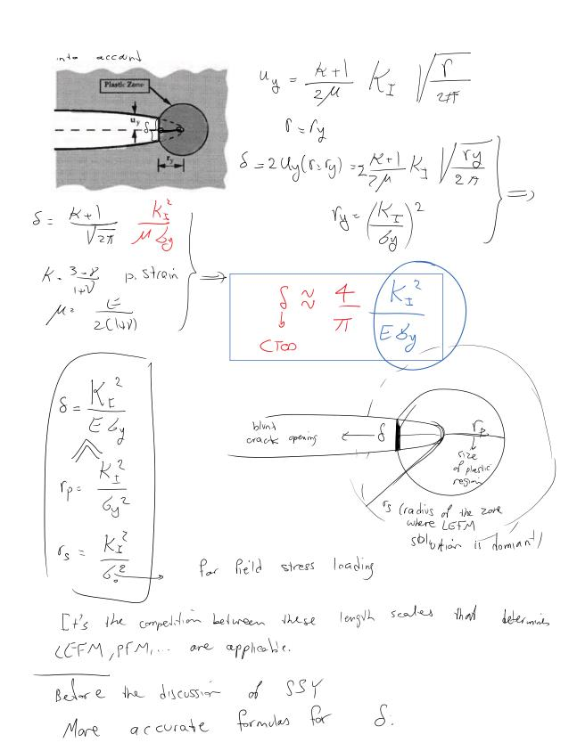
Strip yield model that takes stress redistribution into account on the crack line provides a more accurate estimate for CTOD:
