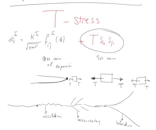
crack a Torress / cract oscillate less & its path be comes more stable! side note How about the effect of T stress crack growth, taughness JyJ d better for yielding toughness toughness / if want to use T stress tranclify ) - reduce
