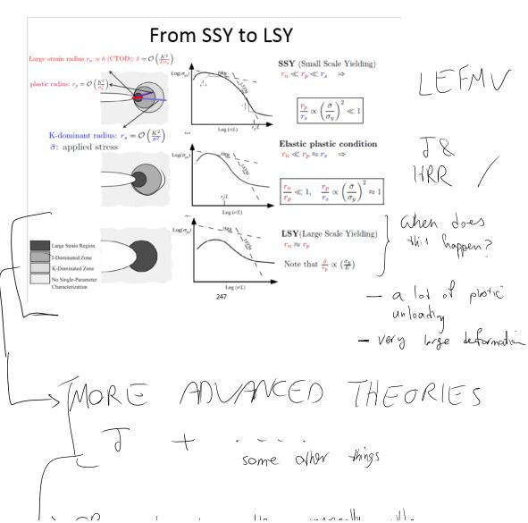
Solve the problem numerically with plasticity, large abormation. From SSY to LSY **LEFM: SSY satisfied and generally** have Generally have  $\bar{\sigma} \ll \sigma_y$ Relevant parameters: G (energy) K (stress) PFM (or NFM): SSY is gradually violated and HRP  $\bar{\sigma} \approx \sigma_y$ Relevant parameters:
