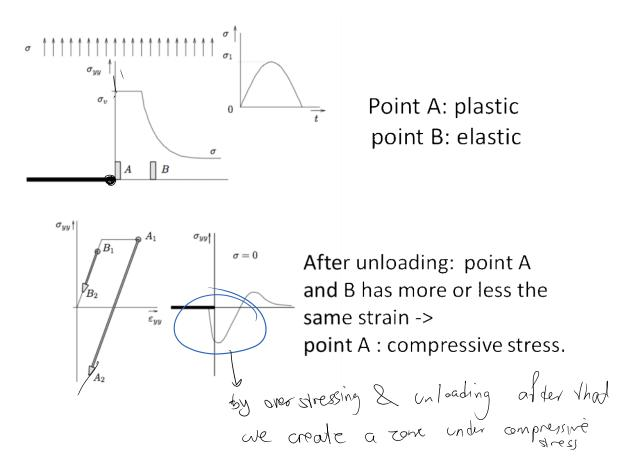
It was recognized empirically that the application of a tensile overload in a constant amplitude cyclic load leads to crack retardation following the overload; that is, the crack growth rate is smaller than it would have been under constant amplitude loading.
