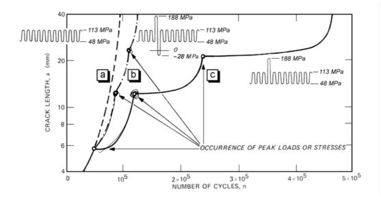
Putting material in compressive stress state is a good idea to retard fatigue crack growth
