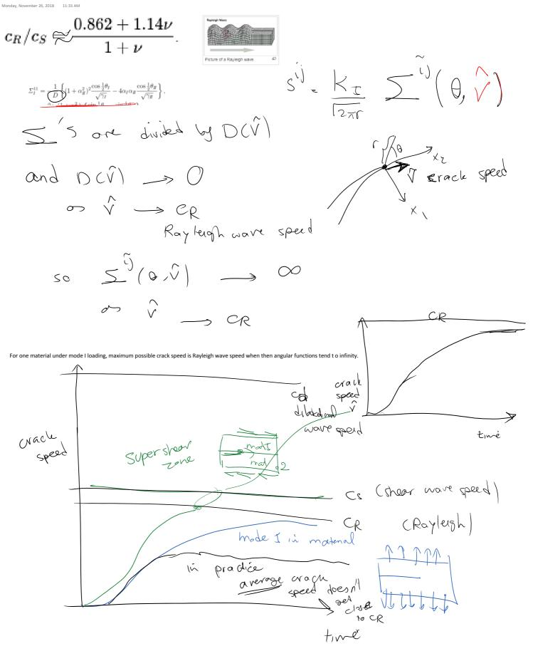
Steps for solving a dynamic LEFM problem 1. K =? wheel is stress intensity factor equal to? I or 1 for mode I I ~ 2 " " [ exampter to j ĵ ĵ ĵ ĵ ĵ ĵ ĵ ĵ infinite demain for example we want to calalate Kal this Inè  $k_{k}(t, \alpha, V) =$ lower shest hym stress KK, (V) K(K, (t,a, 0) tode on lower surres quasi-static Zero crack Bastcally get K(K) (+,a,c) problem speed
