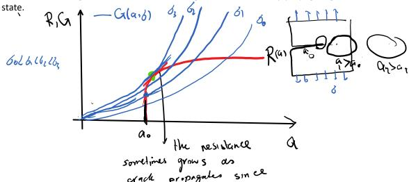
crack propagates since plastic field around crack tip fully develops
