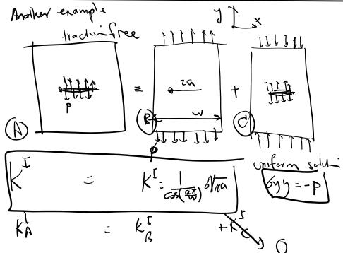
Internal pressure is generally exerted from a fluid. Some examples are hydraulic fracturing, pressure vessel fracture, porous media, ...
