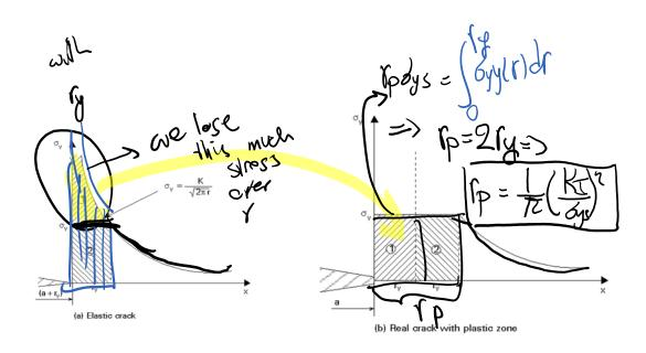
To get the actual process zone size, we need to solve the problem (BC + PDE + constitutive equations) from the beginning to find the correct solution for that problem. The stress solution for the exact problem is NOT the same as LEFM solution even outside r\_p and LEFM stress solution is distributed.
