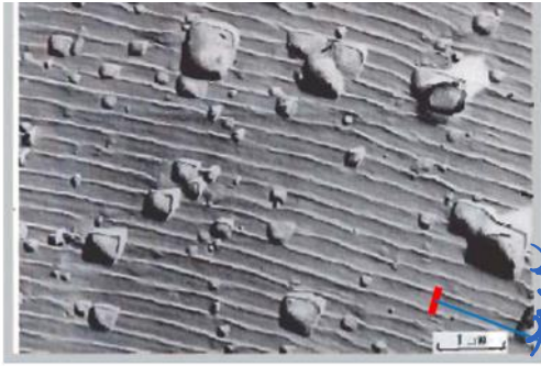
Fracture surface of a 2024-T3 aluminum alloy (source S. Suresh MIT)
