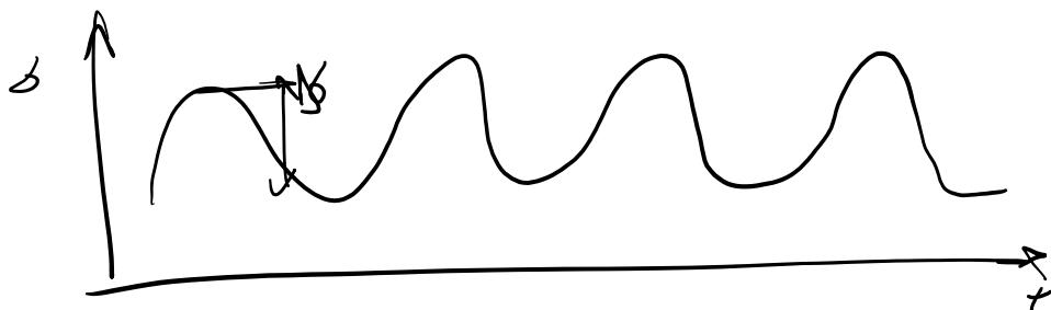
$$\frac{dN}{da} = C(\Delta k)^m = C \left( \pi^{\frac{k}{2}} \Delta \delta^{\frac{k}{2}} a^{\frac{k}{2}} \right)^m$$
