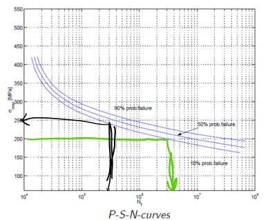
Work with 10% prob of failure
