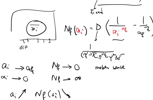
As shown below, ai has a significant influence on Nf (number of cycles to failure):
