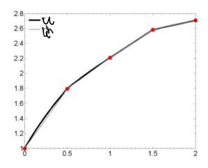
•  $u^h$  and u match at all nodes  $n_0, n_1, n_2, n_3$ , and  $n_4$ . This holds for 1D solid elements with uniform AE and does not hold in general.
