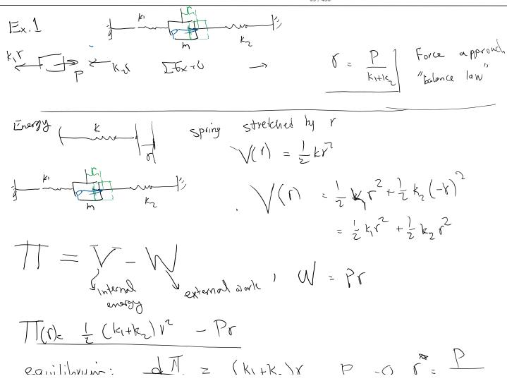
$\frac{d\pi}{dr} = (k_1 + k_2)r - P$   $\frac{d^2\pi}{dr} = k_1 + k_2 > 0$ 17(1) Pol. Energy for a T = V-W  $V = \int_{-2}^{1} EIy^2 dx$ 2W = (3F) y 29 dx) y With the harrow partial boundary  $W_{\Gamma} = \int_{-\infty}^{\infty} dW = \int_{-\infty}^{\infty} (9dx) y = \int_{-\infty}^{\infty} 9y dx$ Mg = - Vg(L) + M g'(L) The Stelly dx-(VyC)+my(L)-Syldx P13 20 779 V-W= ( = Ety'dx - Jygdx
