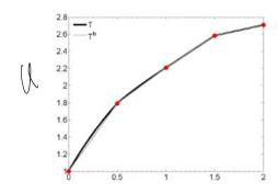
•  $u^h$  and u match at all nodes  $n_0, n_1, n_2, n_3$ , and  $n_4$ . This holds for 1D solid elements with uniform AE and  $\underline{does\ not\ hold}$  in general.
