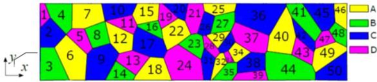
FIGURE 13. The location of 50 grains of materials A, B, C, D in a square domain.
