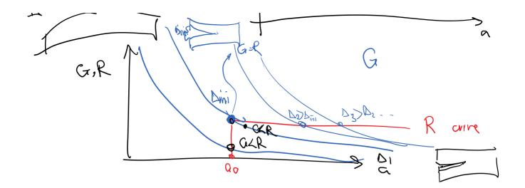
We need to increase the applied displacement  $\triangle$  for the crack to continue propagation -> stable crack growth
