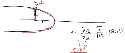
The real crack opening is like:
