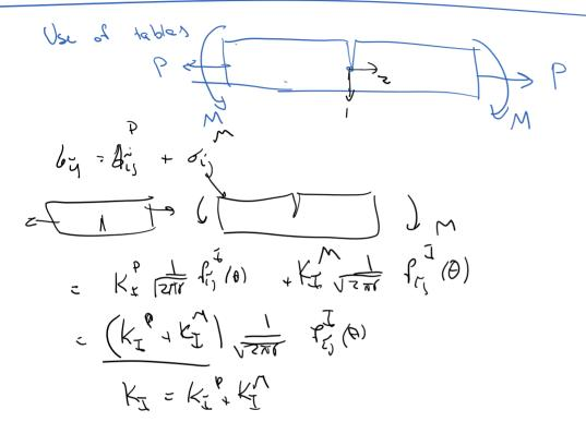
Determine the stress intensity factor for an edge cracked plate subjected to a combined tension and bending.
