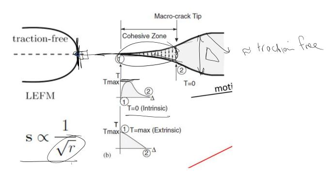
Cohesive models eliminate the singularity of the stress and strain fields around the crack tip
