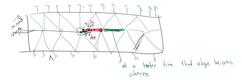
We can do similar fragmentation problems with extrinsic models, but handling the mesh connectivity and interactive insertion of cohesive surfaces is more difficult.
