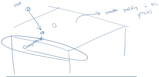
A typical residual stress profile created by shot peening is shown
