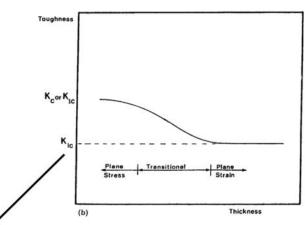
Plane strain fracture toughness lowest K
