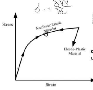
Monotonic loading: an elastic-plastic mate is equivalent to a nonlinear elastic material
