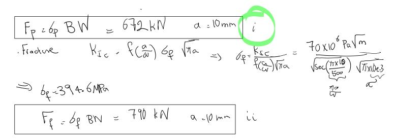
The specimen will fail by yielding for a = 10 mm.
