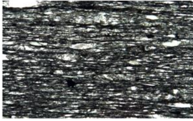
anisotropy in a metamorphic slate. (M. Ismael et. al. 2017)
