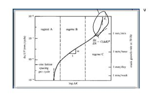
Enal point: in AK we only need to consider K's that are possive & crack is open
