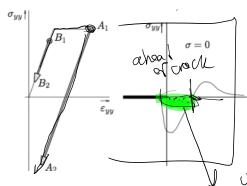
After unloading: point A and B has more or less the same strain ->
